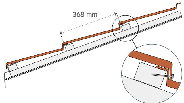
The panels are placed onto battens spacing 368 mm.
